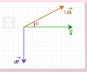
The direction of force when current element i.dL and B are perpendicular to each other can also be determined by applying either of the following rules:
