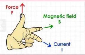
2 Right-hand Palm rule: Stretch the fingers and thumb of the right-hand at right angles to each other. To find the direction of the magnetic force on a positive moving charge, the thumb of the right hand ponts in the direction of velocity of particle v, the fingers in the direction of Magnetic Field B, then the Force F is directed perpendicular to the right hand palm
